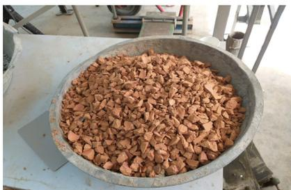
Figure 2: Clay brick aggregate
