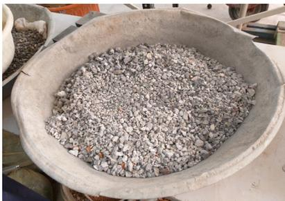
Figure 1: Recycled concrete aggregate
