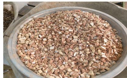
Figure 3: crushed ceramic aggregate
